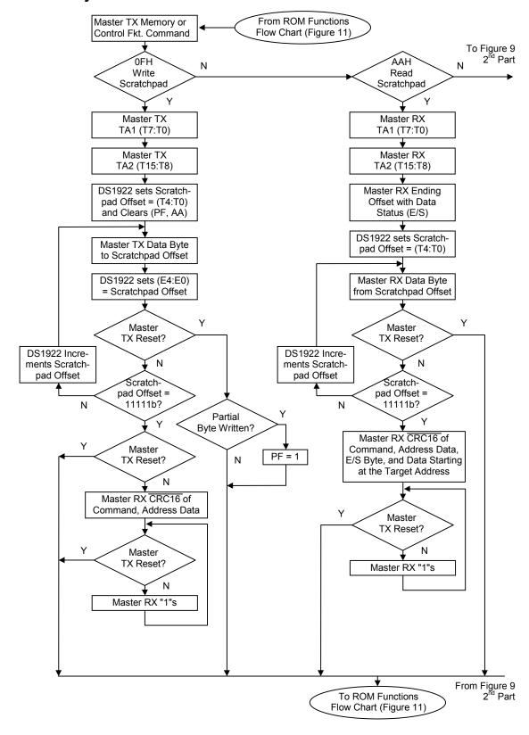
Figure 9-1. Memory/Control Function Flow Chart
