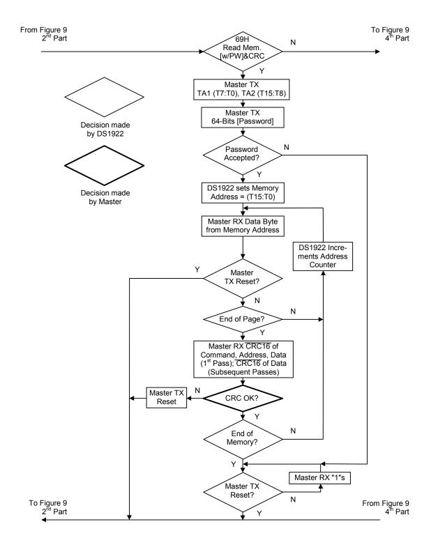
Figure 9-4. Memory/Control Function Flow Chart
