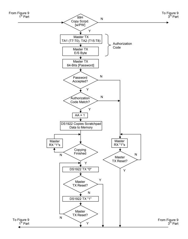
Figure 9-3. Memory/Control Function Flow Chart
