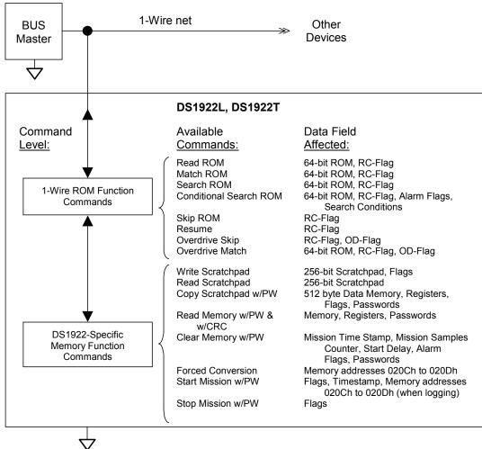
Figure 2. Hierachical Structure for 1-Wire Protocol
