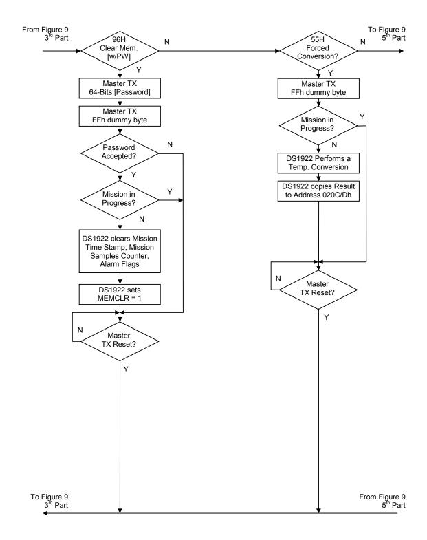
Figure 9-5. Memory/Control Function Flow Chart
