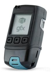
This stand-alone data logger measures and stores over 250,000 temperature and humidity readings over a -30 to  $80^{\circ}$ C (-22 to  $176^{\circ}$ F) and 0 to  $100^{\circ}$ RH range at a resolution of  $0.1^{\circ}$ C ( $0.1^{\circ}$ F) and  $0.1^{\circ}$ RH.
